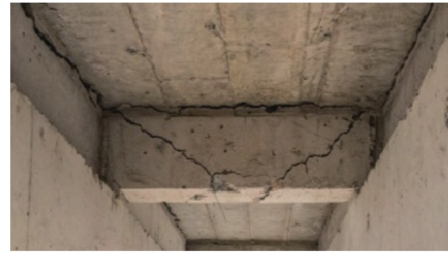
图10 水下爆炸下横梁的破坏效应 Fig.10 Damage effects of crossbeam by underwater explosion
