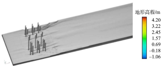
图 12 桩群冲刷后三维地形高程分布 Fig. 12 Elevation distribution of three-dimensional topography after pile scouring
