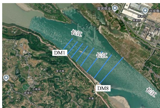
图5 油榨碛滩段雷达测流断面布置 Fig. 5 Layout of radar hydrometric survey cross-section at Youzhaqi section
