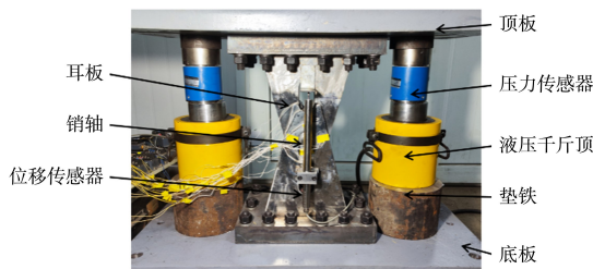
图 3 承载力试验加载装置 Fig. 3 Loading device for load-bearing capacity experiment
