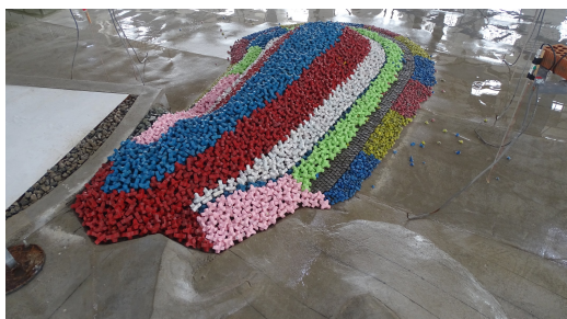
图9 防波堤堤根段稳定情况 Fig.9 Stability of breakwater root
