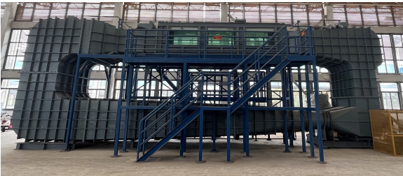
图 4 循环水槽 Fig. 4 Circulating flume
