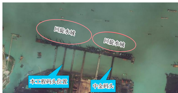
图4 码头回旋水域与周边码头回旋水域关系 Fig.4 Relationship between turning water areas of the terminal and surrounding terminal
